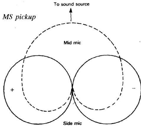
But as with any coincident pair of microphones, their ability to preserve the stereo image in the final mix is the contentious issue among the film post-production fraternity. In XY or MS pairs, any common signal - or signal which arrives at both microphones at the same time (in phase) - can't easily be decoded by Dolby Stereo processing in the final mix and these in-phase signals tend to collapse into the centre speaker.
